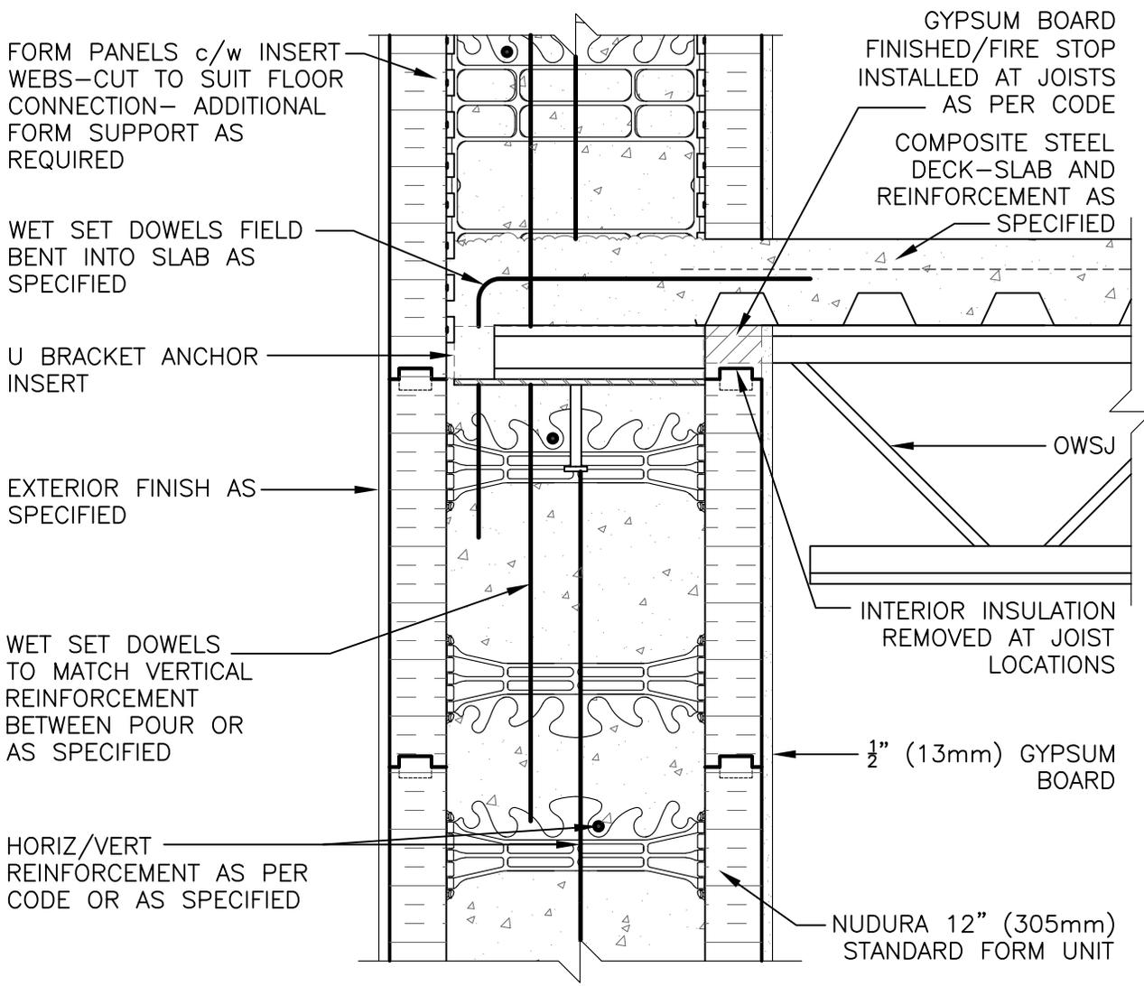
FORM PANELS c/w INSERT WEBS—CUT TO SUIT FLOOR CONNECTION— ADDITIONAL FORM SUPPORT AS REQUIRED
